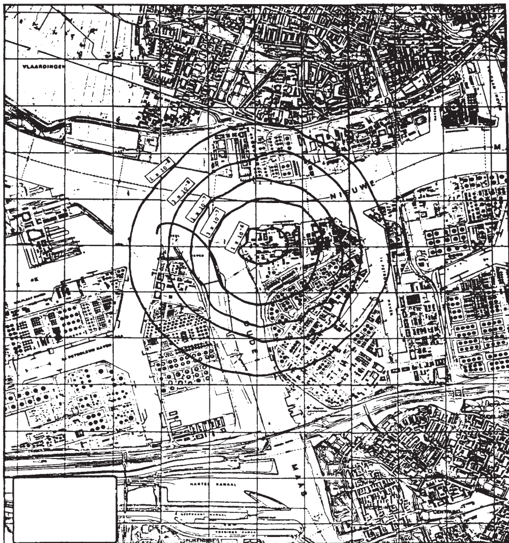
Figure A8.4 Rijnmond Report: risk contours for ammonia storage (Rijnmond Public Authority, 1982. Reproduced by permission)
